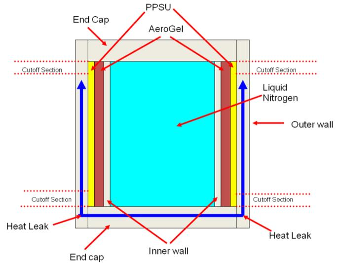
Figure 4 – Alteration to tank
