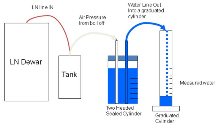
Figure 2 - Clausius-Clapeyron Test Setup
